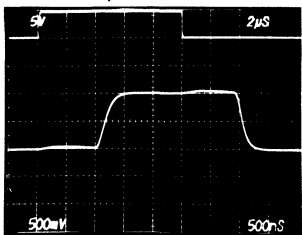
SMALL SIGNAL SWITCHING WITH FILTERING AND 2.5μS SAMPLE TIME
