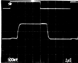
MUX-24 SMALL SIGNAL SWITCHING WITH FILTERING
